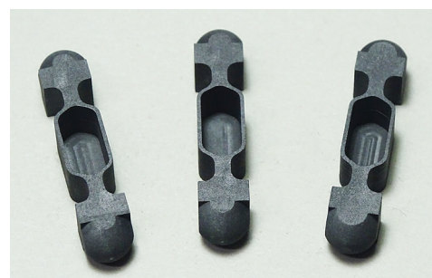
Progression of crucible designs through to the practical and highly successful German designed large volume crucible.
